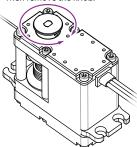
(5) Pushing the switch button forward will keep the spool unlocked.
