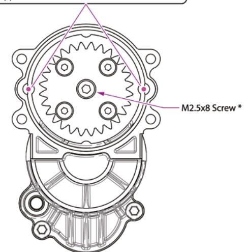
\*To install the spur gear, install the four M2x5 screws, then the center M2.5x8 screw.
