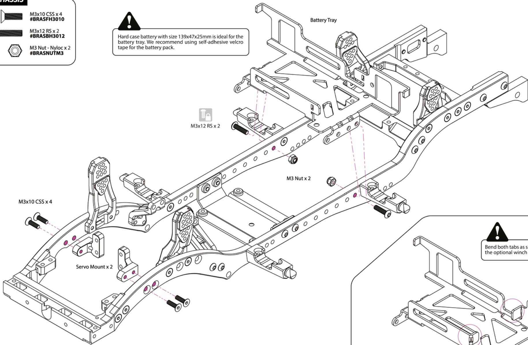
The battery tray is designed to fit a standard size servo winch if you wish to install one. A smaller sized battery pack is required to provide enough space to do so (maximum 95x47x25mm).
