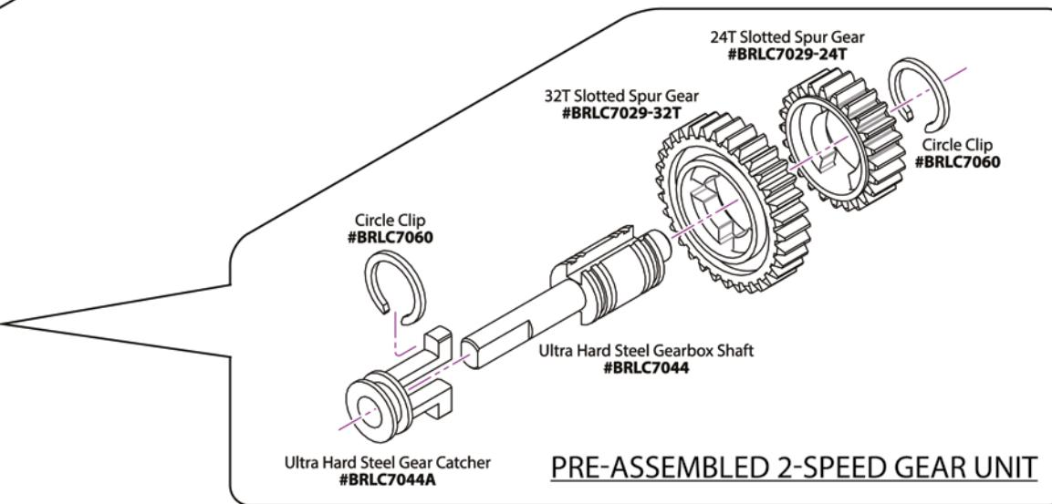
PRE-ASSEMBLED 2-SPEED GEAR UNIT
