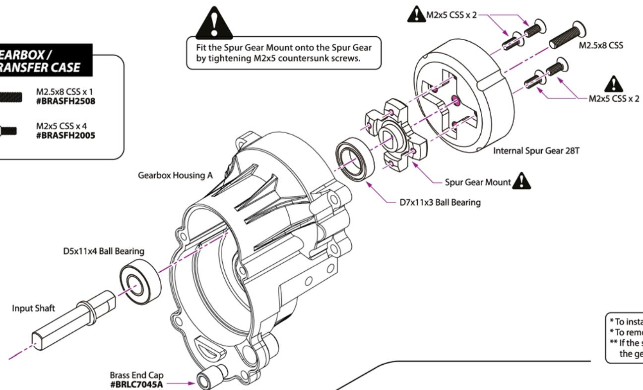
To install or remove the spur gear from the gearbox, align the spur gear as pictured and temporarily insert two M3 screws\*\* to act as stoppers.
