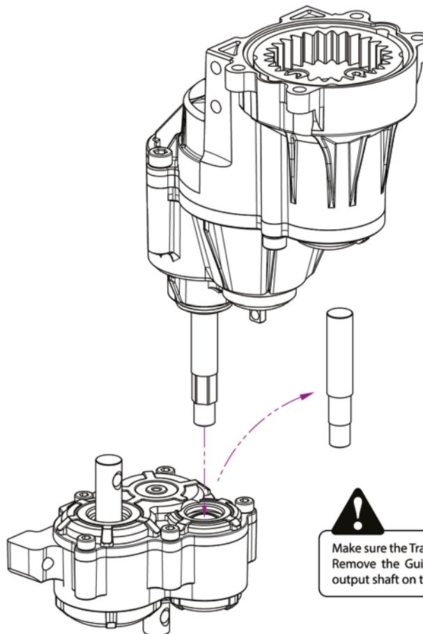
Make sure the Transfer Case is kept in the upwards position.
