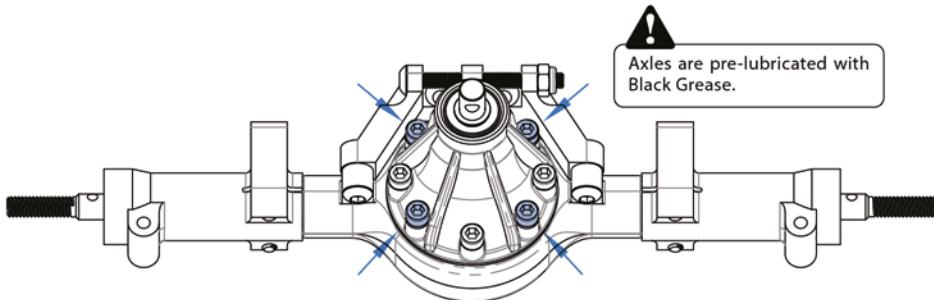
Step 1 - Loosen four M2.5x16mm socket screws indicated making the screw cap 3 mm apart from the case.
