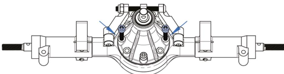
Step 1 - Remove all M2.5x16mm and two M2.5x5mm socket screws
