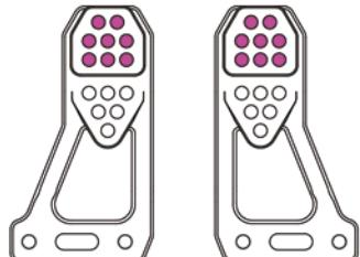
Only use highlighted holes as optional damper installation position to increase chassis ground clearance.
