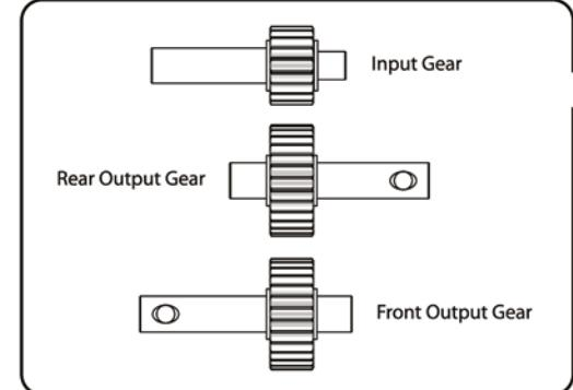
Apply black grease on the teeth and both sides of the input gear to avoid spacers misaligned when connecting to the gearbox.
