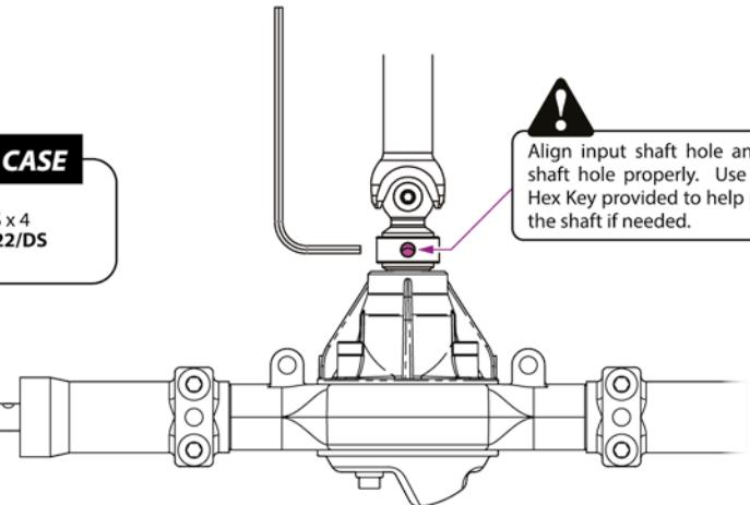
Align input shaft hole and drive shaft hole properly. Use the 1.5 Hex Key provided to help pull out the shaft if needed.
